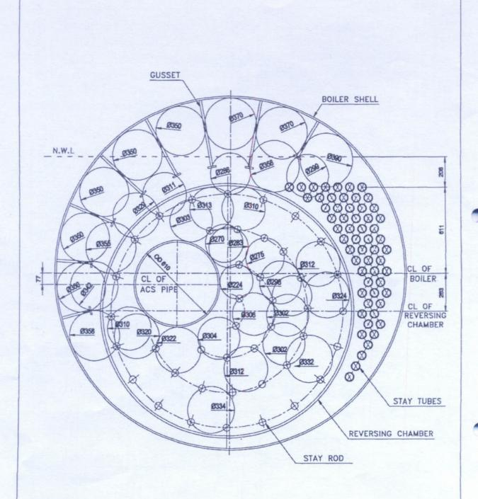
PRESSURE CIRCLE DIAGRAM FOR SHELL REAR END PLATE
